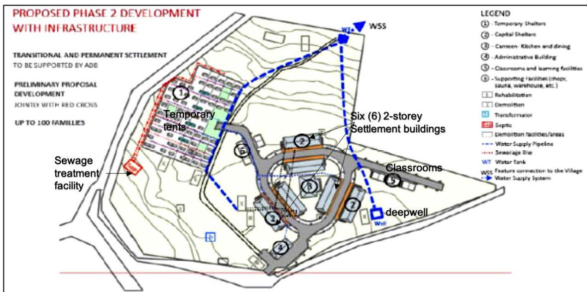
Figure 3: Preliminary site development plan of Phase 2
